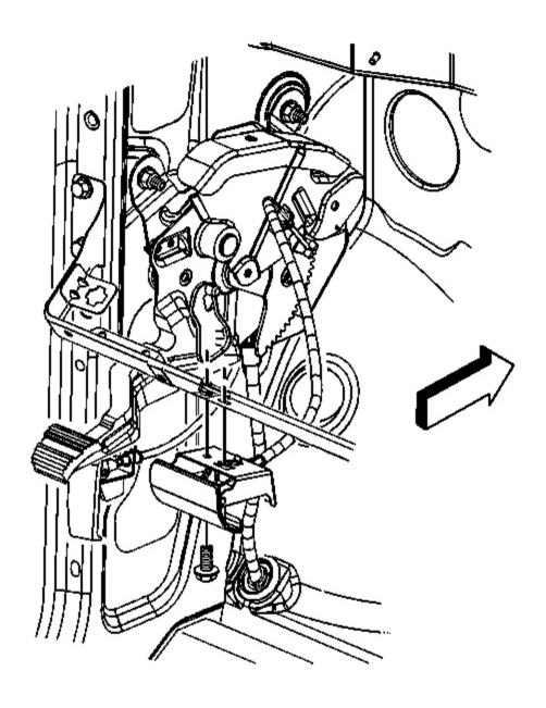
Fig. 7: Park Brake Release Lever Handle & Bolt Courtesy of GENERAL MOTORS CORP.
