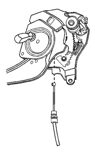
Fig. 12: Front Park Brake Cable & Park Brake Lever Courtesy of GENERAL MOTORS CORP.
