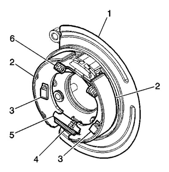
Fig. 2: Park Brake Shoe Return Springs Courtesy of GENERAL MOTORS CORP.
