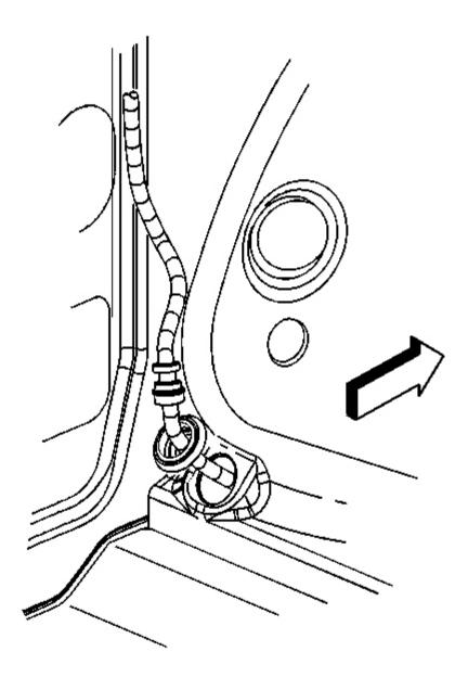
Fig. 21: Access Cable Grommet Courtesy of GENERAL MOTORS CORP.
