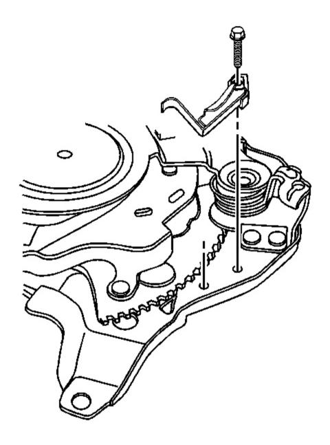
Fig. 18: Park Brake Warning Lamp Switch Courtesy of GENERAL MOTORS CORP.
