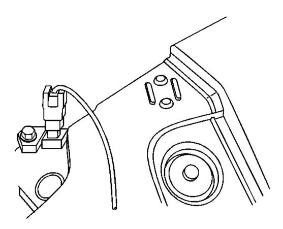
Fig. 17: Park Brake Warning Lamp Connection Courtesy of GENERAL MOTORS CORP.
