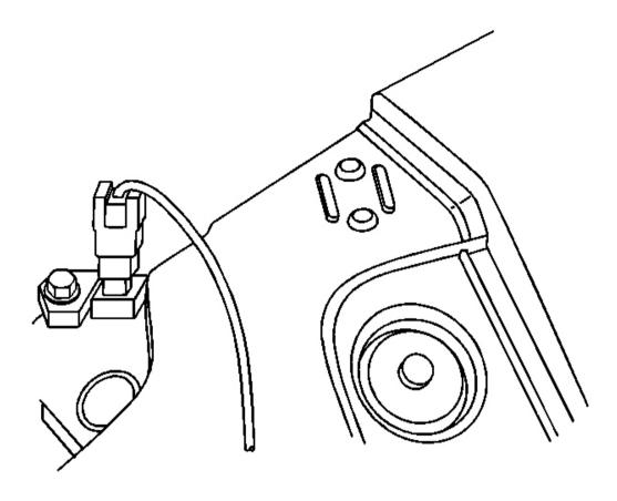
Fig. 16: Park Brake Warning Lamp Connection Courtesy of GENERAL MOTORS CORP.
