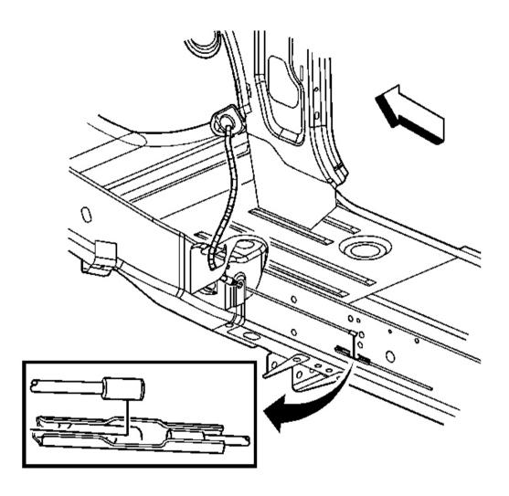
Fig. 22: Front/Intermediate Park Brake Cable Courtesy of GENERAL MOTORS CORP.
