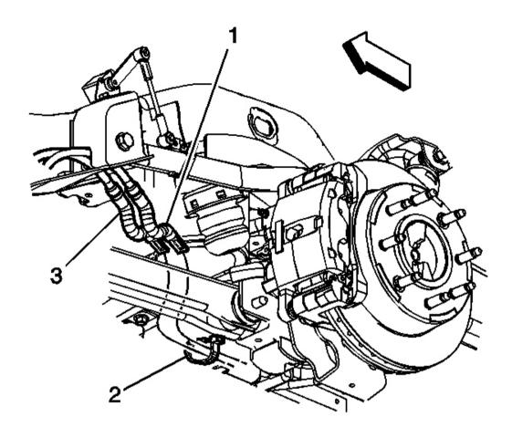
Fig. 39: Right Rear Cable & Cable Guide Courtesy of GENERAL MOTORS CORP.
