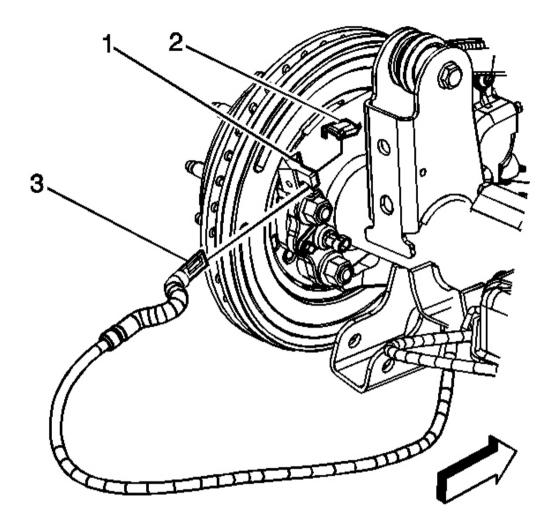
Fig. 6: Cable, Lever & Backing Plate Courtesy of GENERAL MOTORS CORP.
