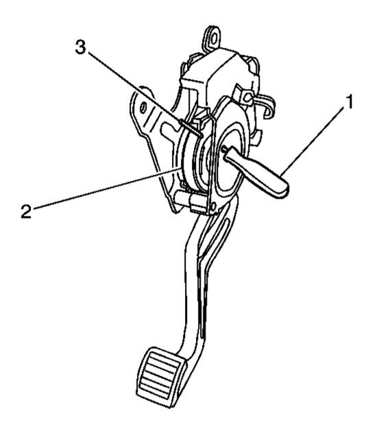
Fig. 48: Park Brake Cable Automatic Adjuster Courtesy of GENERAL MOTORS CORP.
