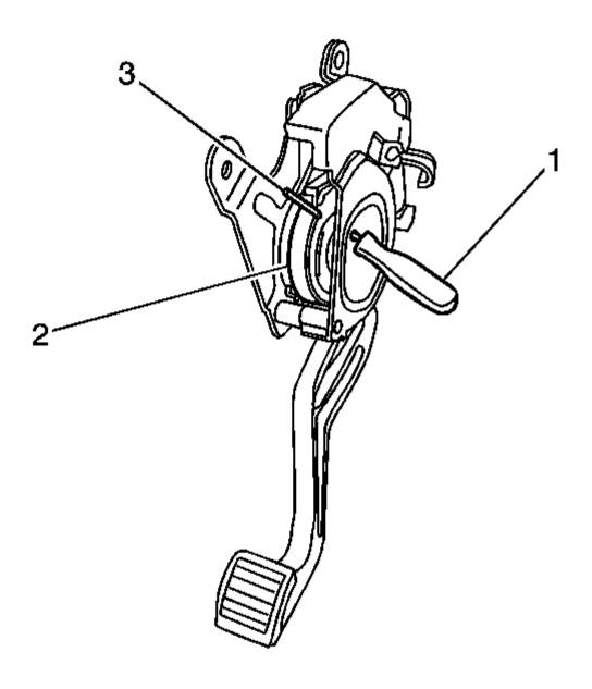
Fig. 49: Park Brake Cable Automatic Adjuster Courtesy of GENERAL MOTORS CORP.
